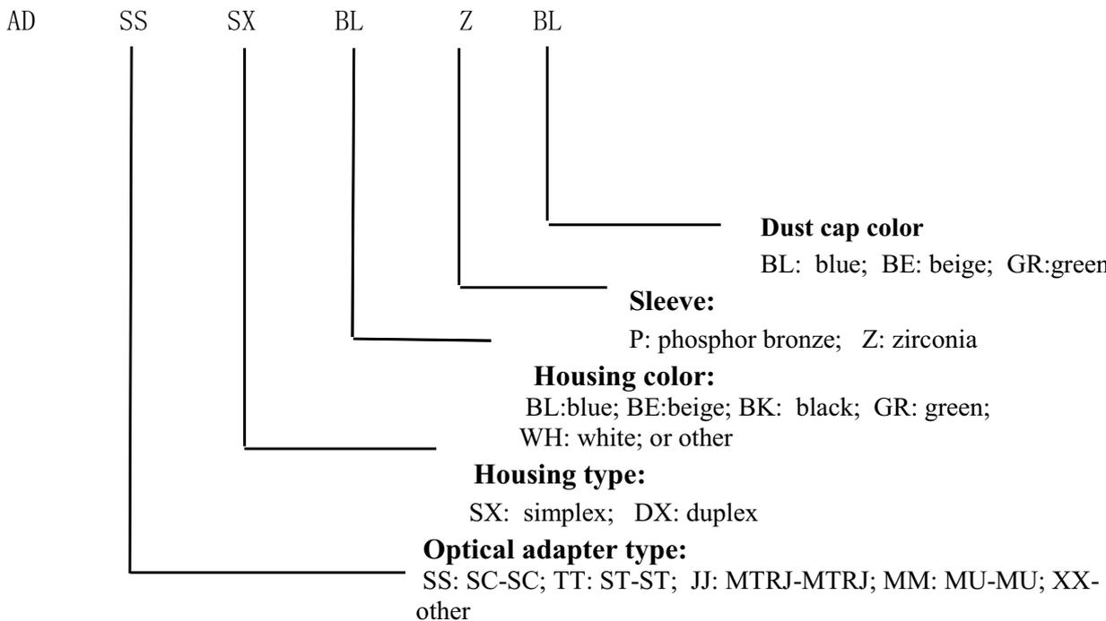
Example: ADSSXBLZBL: Denotes adapter,SC-SC simplex type,zirconia sleeve,blue housing and dust cap
